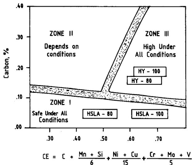
Fig. 1 Weldability of steel as a function of carbon content and carbon equivalent from Graville (Ref 9)
