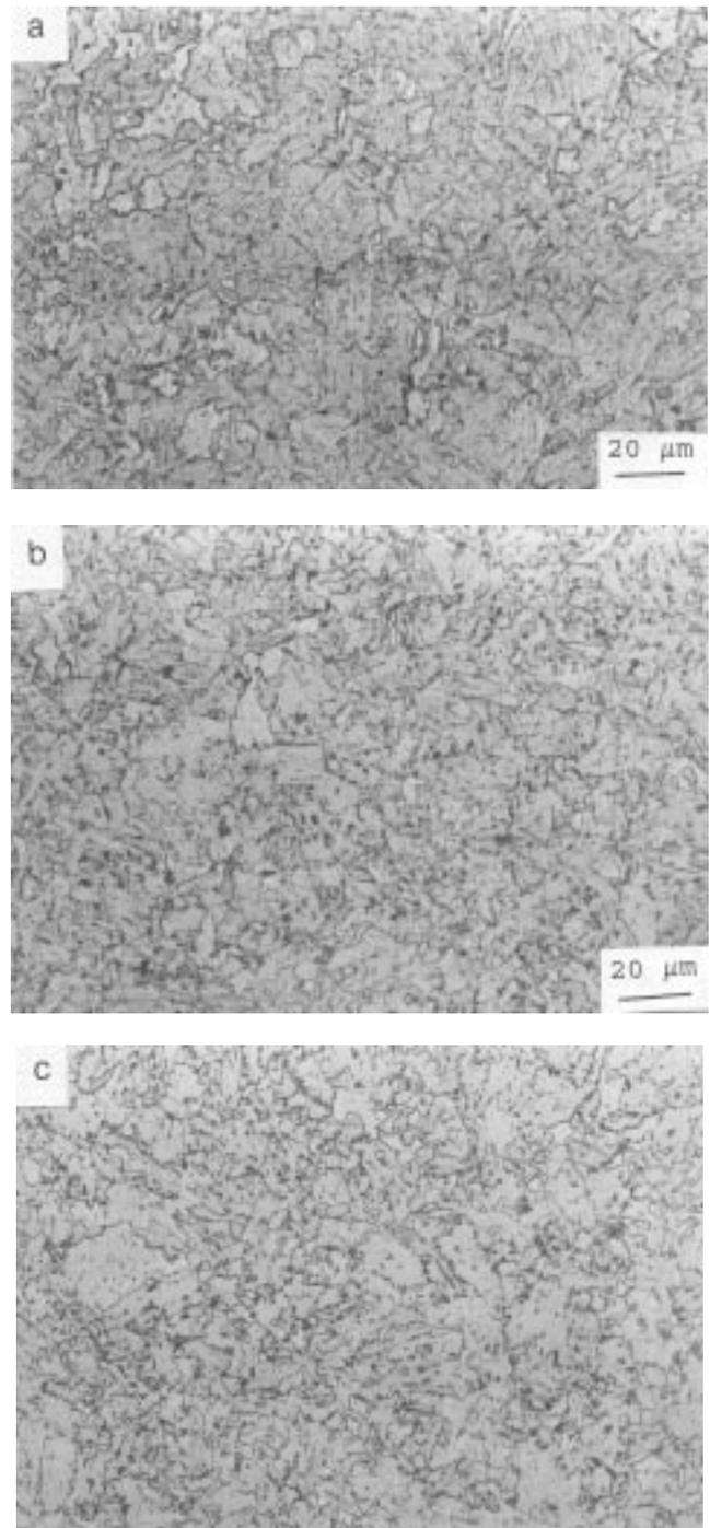
Fig. 2 Optical micrographs showing acicular ferrite in HSLA steel plates. (a) 12 mm thickness. (b) 14 mm thickness. (c) 16 mm thickness. 500 $\times$  (Art has been reduced to 83% of its original size for printing).
