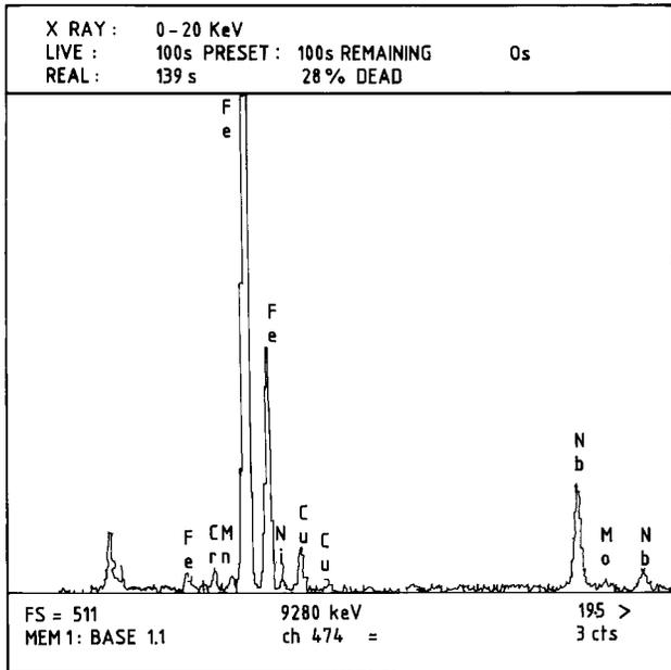
Fig. 5 EDS spectrum of niobium-rich particles in Q&T plates of the production HSLA steel
