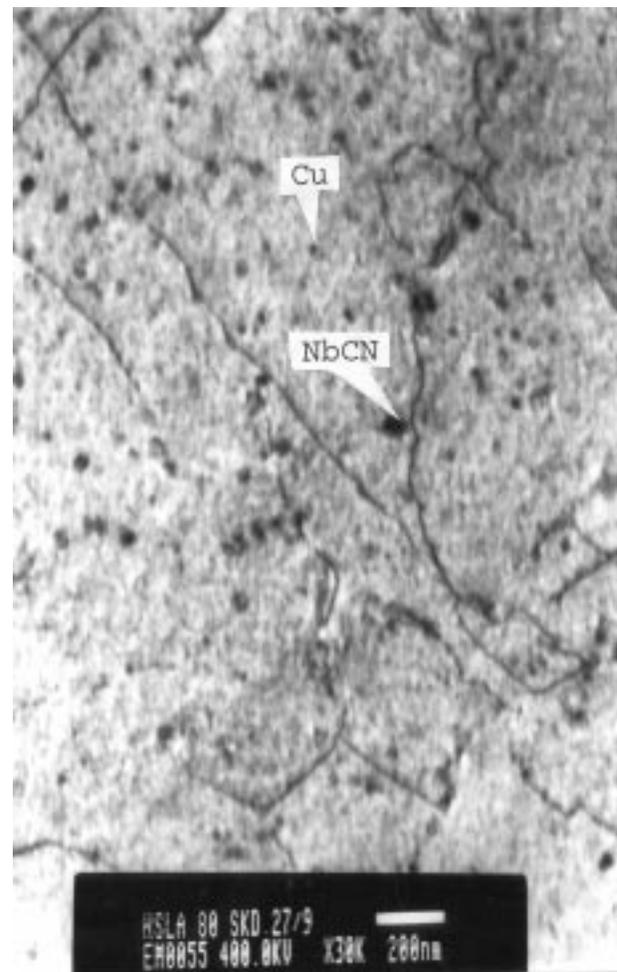
**Fig. 4** Bright-field TEM image of thin-foil specimen from 14 mm thick quenched-and-aged HSLA steel plate showing copper precipitates. 30,000×
