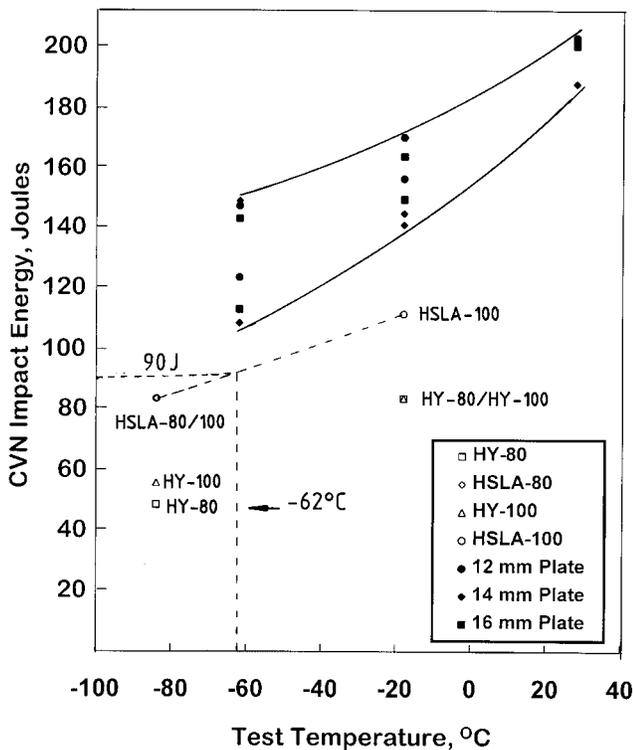
Fig. 6 Variation of CVN impact energy with temperature in transverse specimens of HSLA steel plates
