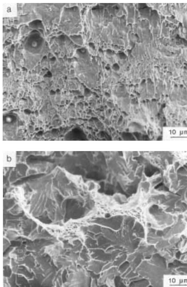
**Fig. 7** SEM fractograph of Charpy impact specimen tested at  $-62$  °C showing (a) ductile features near notch and (b) brittle cleavage region slightly away from notch. 1000 $\times$  (Art has been reduced by 80% for printing).
