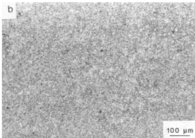
**Fig. 3** Optical micrographs showing fine-grained acicular ferrite in HSLA steel plates. (a) 12 mm thickness. (b) 14 mm thickness. 100× (Art has been reduced to 83% of its original size for printing).
